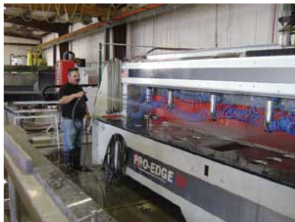
In 2004, Stone Concepts added a Pro Edge III automated edging machine from Park Industries.
