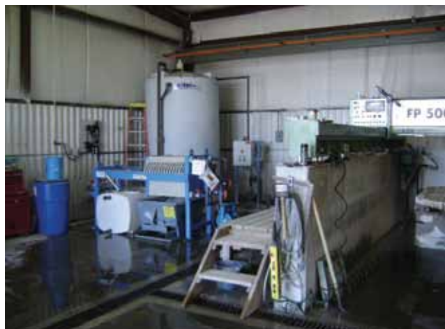
Water is recycled using an EnviroSystem from Water Treatment Technologies.
