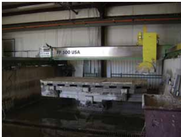
One of the shop's first investments was a FP 500 bridge saw from Simec of Italy.
